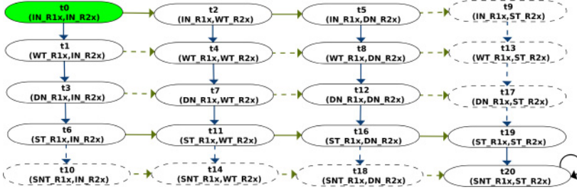
Fig. 11. Repaired pair-structure for R1x \parallel R2x .
